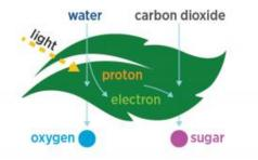
Artificial Leaf | Synthetic leaves have a semiconductor to generate electrons from light, and a catalyst to steal protons from water. These are combined to make hydrogen.
