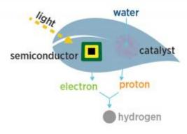
**Bionic Leaf** | These combine lightharvesting tech with microbes. In one design, hydrogen from an artificial leaf is passed to microbes, which then produce useful chemicals.
