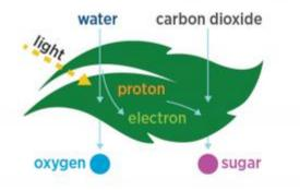
Artificial Leaf | Synthetic leaves have a semiconductor to generate electrons from light, and a catalyst to steal protons from water. These are combined to make hydrogen.
